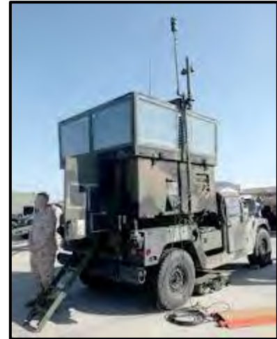
Photo 4.6-1. Expeditionary Control Tower on Humvee
