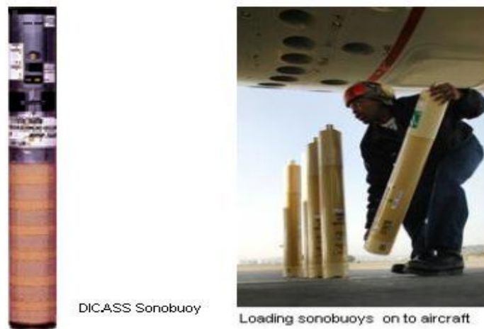
Figure 2.3-3: Sonobuoys (e.g., AN/SSQ-62)
