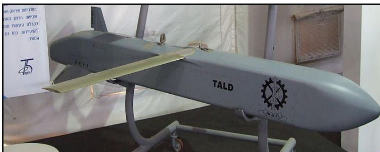
Figure A-3: Tactical Air-Launched Decoy (Aerial Target)
