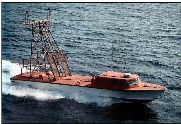
Figure A-5: QST-35 Seaborne Powered Target
