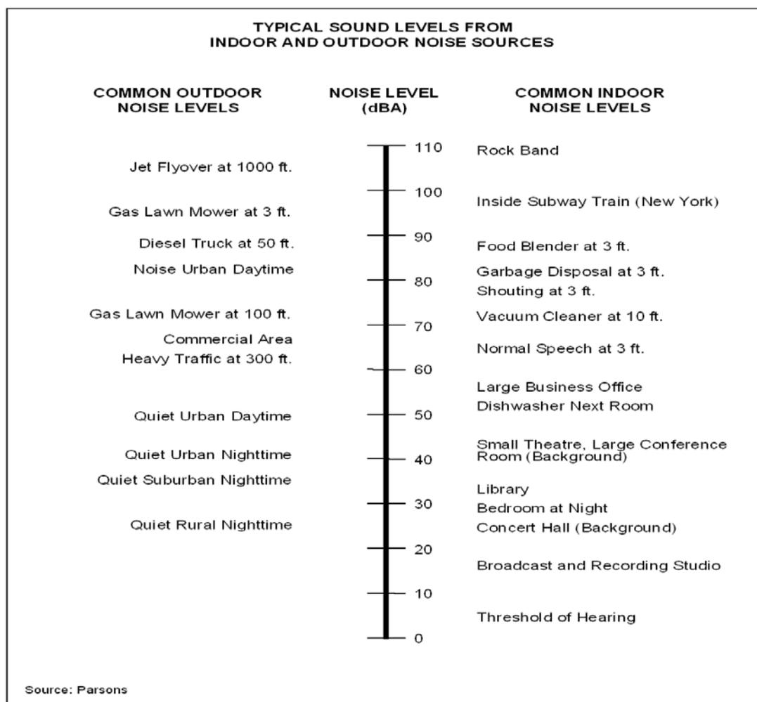
**Figure 6.1-1 Typical A-Weighted Sound Levels of Common Sounds**
